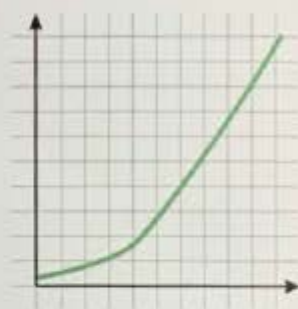
clamping force vs magnetic flux density
