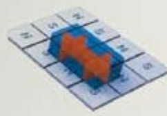
Triple covering 3 north poles, 3 south poles
